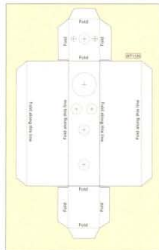
Fig. 4: Dimension for the bracket - which can be formed from aluminium sheet (see text).
