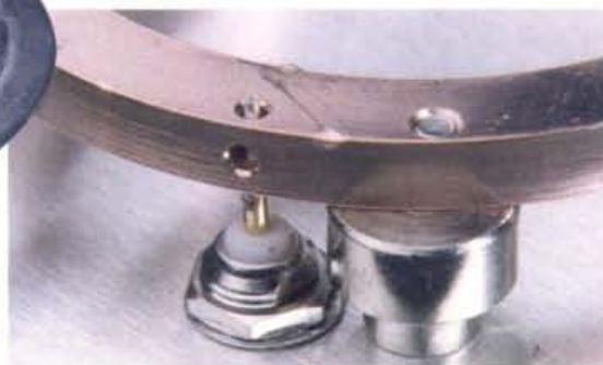
Fig. 2: The feedpoint (on the left) is straight from the BNC plug below. The 'earth' return to the right forms the matching network for the antenna. See text for more detail.
