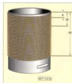
Fig. 3a & b: Coil winding details for the wavemeter project (see text).
