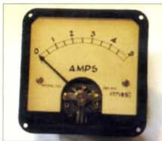
Fig. 1: A 'new lamp' for 'old'! This '5A' full scale deflection (f.s.d.) meter is in fact a 1mA f.s.d. instrument fitted with a 'shunt'. Find out how you can modify moving coil meters yourself, by the use of simple mathematics and a little skill and patience!
