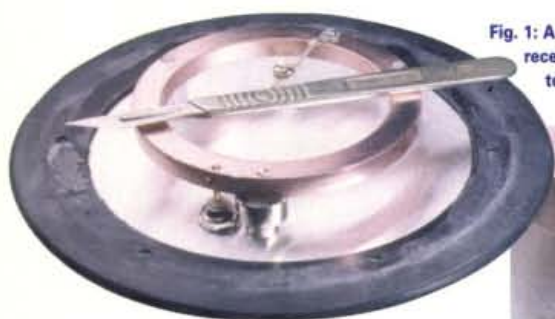
Fig. 2: The feedpoint (on the left) is straight from the BNC plug below. The 'earth' return to the right forms the matching network for the antenna. See text for more detail.
