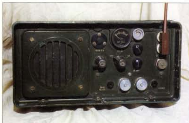
Fig. 1: A B44 military transceiver - ideal for 70MHz operation which was very popular in the early days. (Courtesy of Ben Nock G4BXD - PW 'Valve & Vintage' author).
