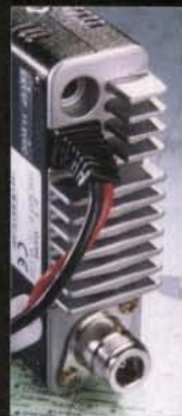
Fig. 1: The rear of the FT-90R. Here you can see the N-type socket (bottom of picture) which Richard mentions in text along with the heat-sink (which is assisted by an internal fan), external speaker socket (top of picture) and power lead.
