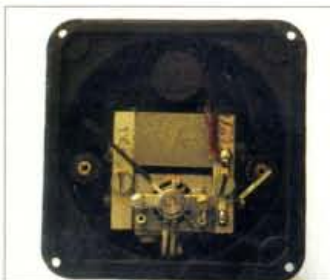
Fig. 2: Once the outer casing has been (carefully!) removed, the meter movement can be seen to advantage. In this example the calibrated scale has also been removed. The magnet can be seen immediately above the 'moving coil' movement, with the (very delicate) aluminium 'needle' pointing towards '10 o'clock'.
