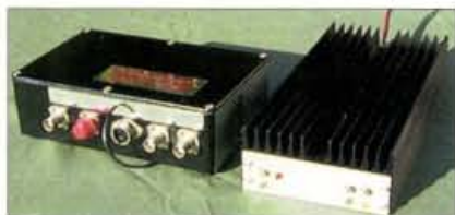
Fig. 3: Derek's microwave module transverter (28-70MHz) can be seen here on the left of the picture with his microwave module 70MHz 100W amplifier (on the right).
