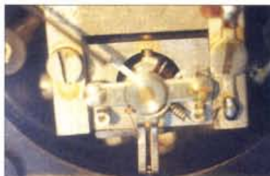
Fig. 3: Close-up of the moving coil meter movement. The parallel 'slotted bar' below the movement is for needle 'zeroing' (this is achieved via an externally adjusted screw-slot mechanism).
