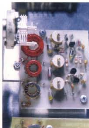
Fig. 3: The Carlton receiver's three-band v.f.o. printed circuit board incorporates toroidal cores, for 3.5, 7 and 14MHz. And although G3XFD says that winding the toroids may provide a challenge, he managed to complete the job!
