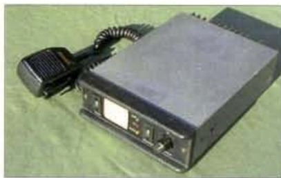
Fig. 4: Derek uses a Tait T199 (made in New Zealand) low-band ex-p.m.r. set for his contacts on the 4m band. He says that these are available from as little as £5 (less crystals) and are easy to modify for 70MHz.
